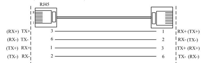
MDI/MDI-X auto connection makes switch easy to use for customers without considering the type of network cable.
