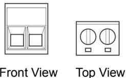
NP302T series provide DC power input, voltage input is the two terminal form, plug type 2 core spacing of 5.08mm terminals, wherein the power input range of 9 ~ 48VDC. (V+, V-)
