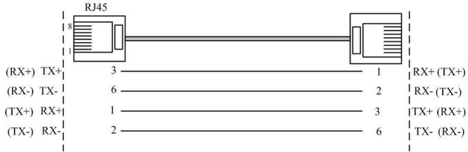
MDI/MDI-X auto connection makes switch easy to use for customers without considering the type of network cable.
