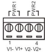
The switch have redundant power input, provides one terminal block (4 bits) for PWR1 and PWR2 input. The redundant power can be used single and used two self-governed power to supply to the system, PWR1 and PWR2 input at the same time, when neither of these two power fails, the other power acts as a backup, and automatically supplies power needs, ensure running Ethernet reassuring. Voltage input range is 12~48VDC (terminal block defined as: V1-, V1+, V2-, V2+).
