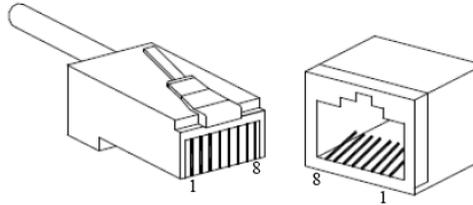
RJ 45 port support automatic MDI/MDI-X operation. That can connect the PC, Server, Converter and HUB. Pin 1, 2, 3, 4, 5, 6, 7, 8 Corresponding connections in MDI. 1→3, 2→6, 3→1, 4→7, 5→8, 6→2, 7→4, 8→5, are used as cross wiring in the MDI-X port of Converter and HUB. In MDI/MDI-X, 100/1000Base-TX PIN defines is as follows:
