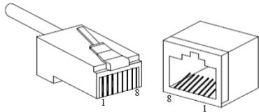
RJ 45 port support automatic MDI/MDI-X operation. Can connect the PC, Server, Converter and HUB .Pin 1,2,3,6 Corresponding connections in MDI. 1→3, 2→6, 3→1, 6→2 are used as cross wiring in the MDI-X port of Converter and HUB. 10Base-T/100Base-TX are used in MDI/MDI-X, the define of Pin in the table as below.
