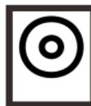
Power supply input: 5VDC, please use DC power adapter: internal diameter, 2.5mm, external diameter, 5.5mm.
