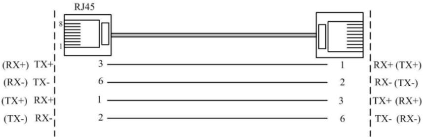
MDI/MDI-X auto negotiation user-friendly IMC102B’s 10/100Base-TX Ethernet interface regardless of the type of Ethernet cable can be directly via crossover cable or straight lines to achieve IMC102B fiber optic transceivers and connection
