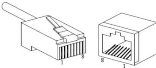
RJ45 port support automatic MDI/MDI-X operation, can connect the PC, Server, Converter and HUB. Pin 1,2,3,6 corresponding connection in MDI.1→3,2→6,3→1,6→2 are used as cross wiring in the MDI-X port of Converter and HUB.10Base-T/100Base-TX are used in MDI/MDI-X, the define of PIN in the table as below.
