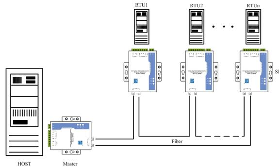
**\*Note:** When loop application, only one Master allow to Master MODEL271, all other Slaves are to Slave MODEL271.
