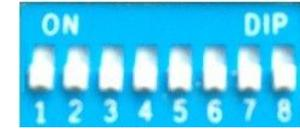
The upper panel of MC201 provides 8 settings of DIP switch for baud rate matching, I/O1 to ON means the user's baud rate setting is valid, otherwise is automatically matched baud rate. 2~6 are status valid values of manually setting baud rate(see table below), 7, 8 as reservation.
