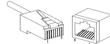
RJ 45 port support automatic MDI/MDI-X operation. Can connect the PC, Server, Converter and HUB .Pin 1,2,3,6 Corresponding connections in MDI. 1→3, 2→6, 3→1, 6→2 are used as cross wiring in the MDI-X port of Converter and HUB. 10Base-T/100Base-TX are used in MDI/MDI-X, the define of Pin in the table as below.
